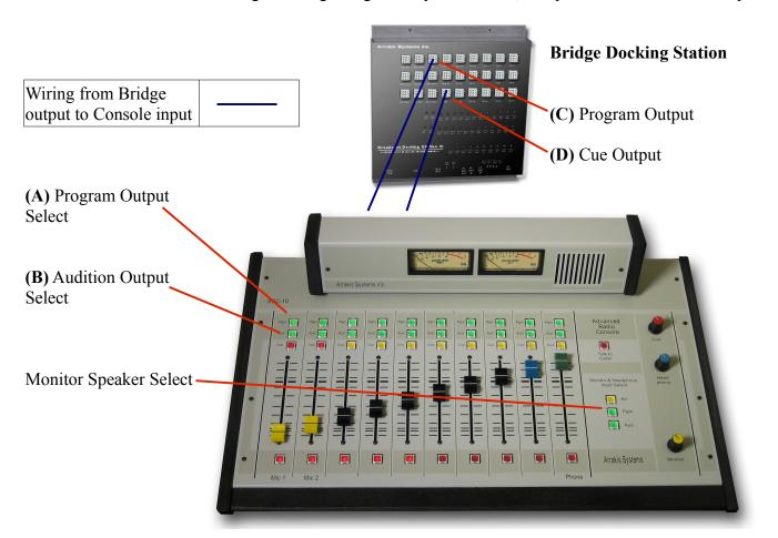
The **(C)** Bridge Program Output and the **(D)** Bridge Cue Output should be connected to 2 different channels on your board. If your console has two outputs (Program & Audition), then every channel on the board has the option of either being played out the **(A)** Program Output or the **(B)** Audition Output. In these instructions, when we refer to the different outputs, it will be notated with the letters from this key:
